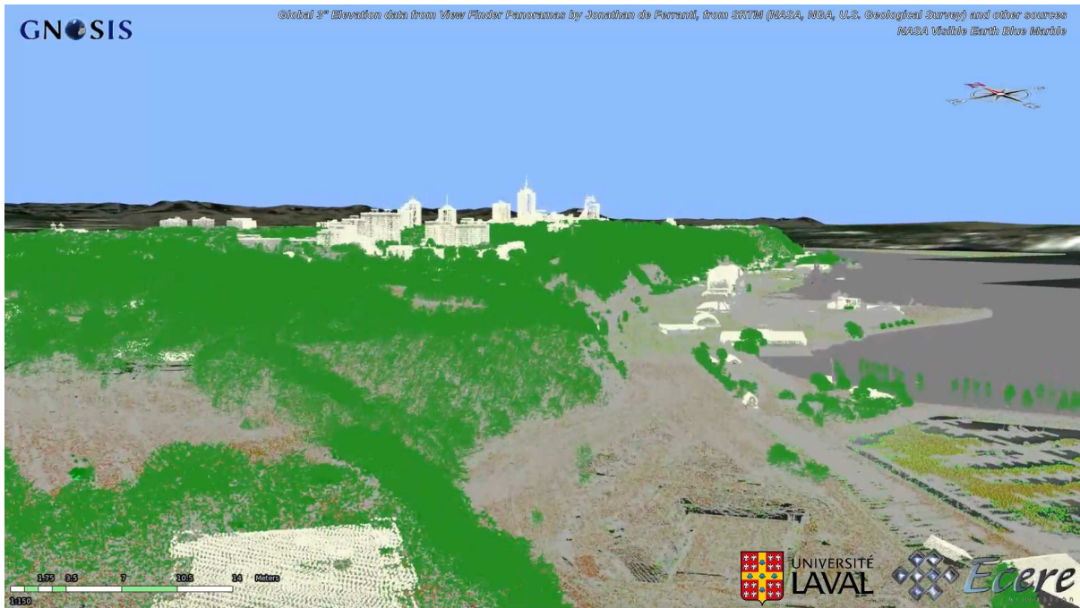
Figure 17. Visualization of classified multi-resolution point cloud (~1 billion points) from LiDAR provided by Université Laval
