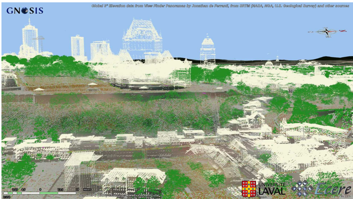
Figure 16. Visualization of classified multi-resolution point cloud (~1 billion points) from LiDAR provided by Université Laval
