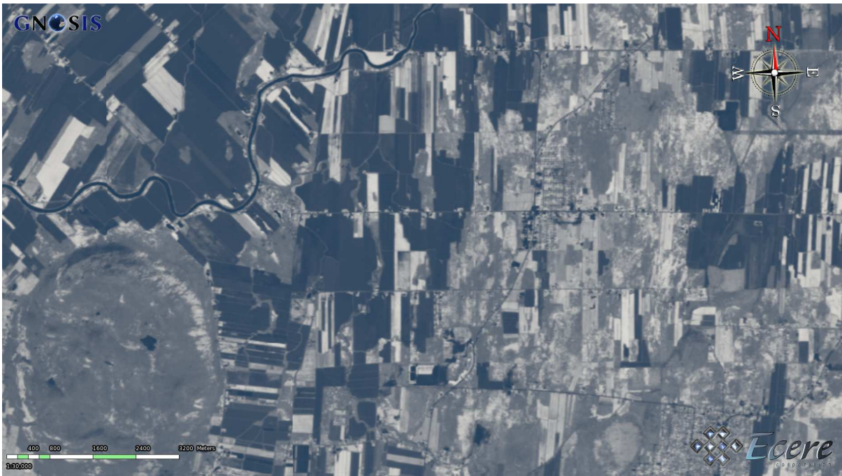
Figure 46. NDVI Calculation performed by javaPS, from sentinel-2 imagery retrieved from EOx's pygeoapi server on the EuroDataCube, accessed via the MOAWAdapter process from GNOSIS Map Server, and visualized in GNOSIS Cartographer
