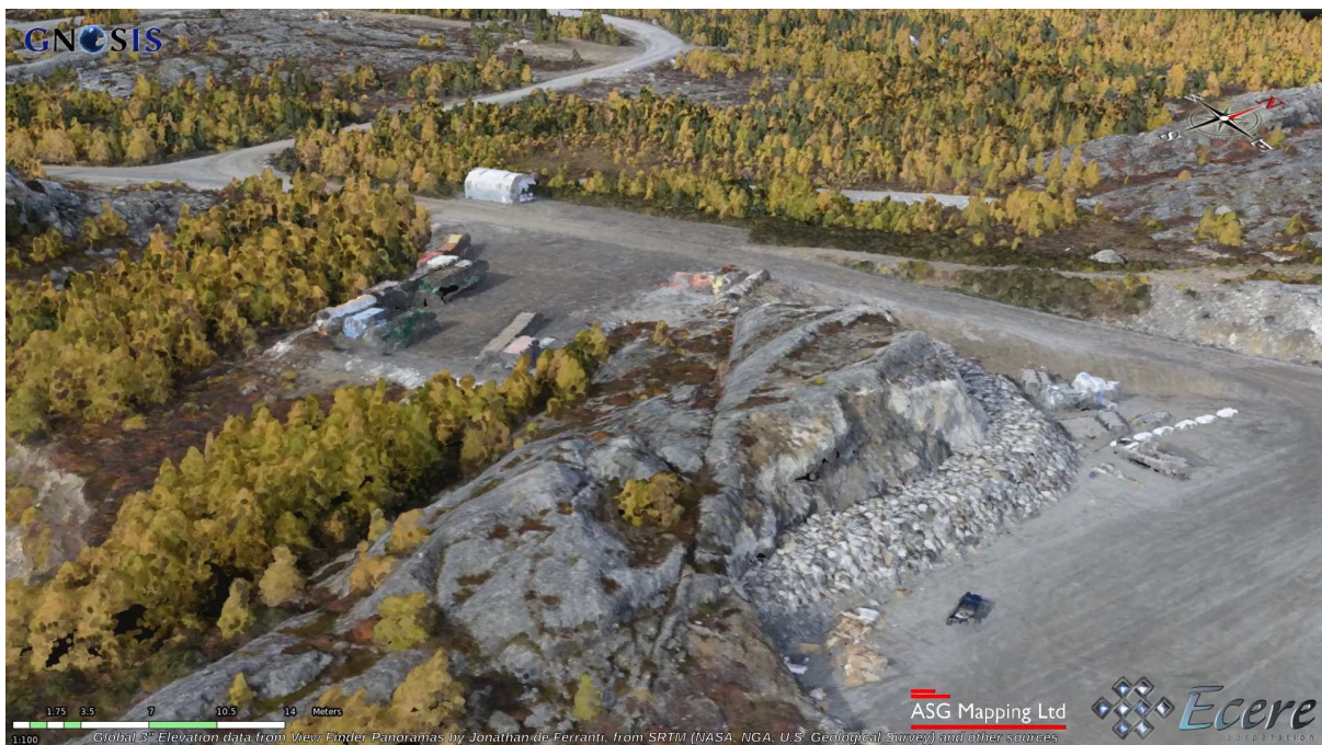
Figure 18. Visualization of multi-resolution point cloud from photogrammetry provided by ASG Mapping, including RGB values
